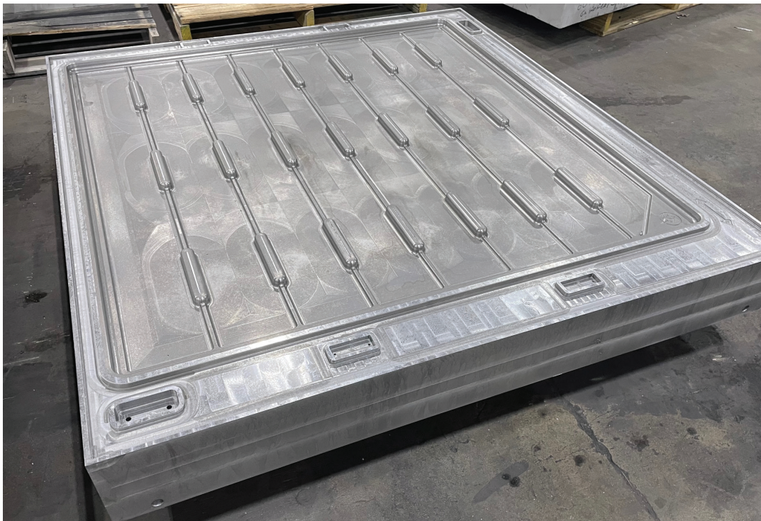
A “cast oversized and machined” mold for a floating dock.
