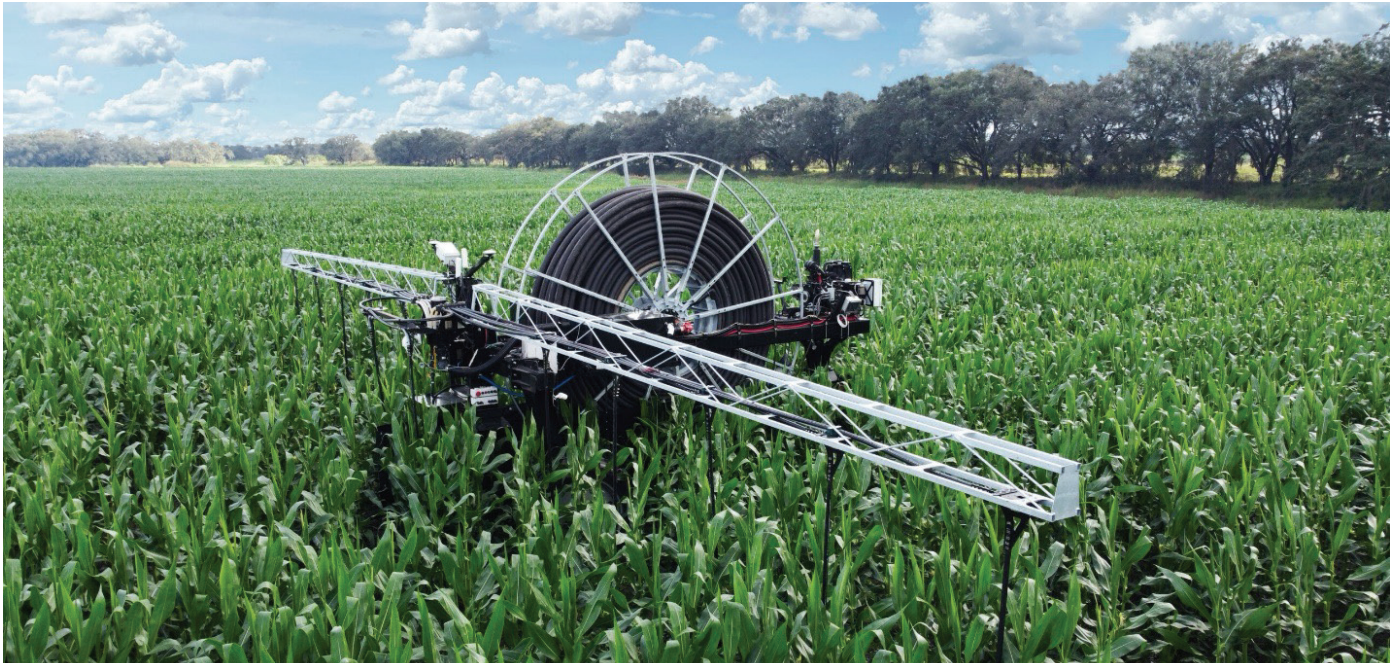
The 360 RAIN delivers bands of water, nutrients, and fungicides directly to the base of plants.
