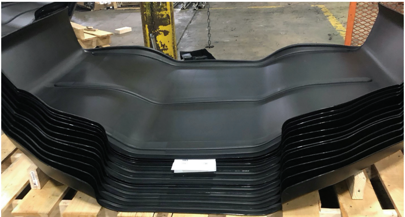
Samples of the new wheel shield thermoformed part.
