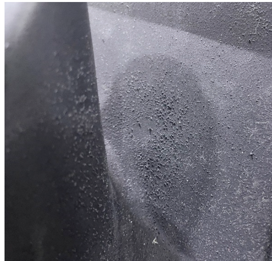
Figure 2 Result of tool porosity on the finished part.
